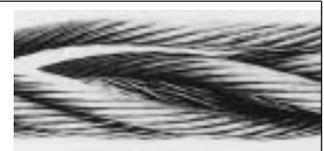
**12** Looped wires as a result of torsional imbalance and/or shock loading.
