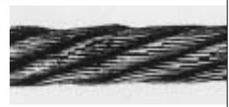
**10** Wire fractures at the strand, or core interface, as distinct from 'crown' fractures.
