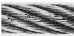
**4** Two parallel paths of broken wires indicative of bending through an undersize groove in the sheave.
