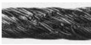
**2** Localised wear due to abrasion on supporting structure.
