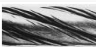
**7** Severe corrosion.
