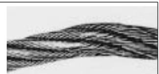
**14** Multi strand rope 'bird caged' due to torsional imbalance.
