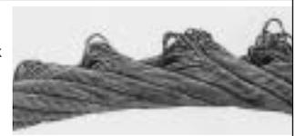
**13** Typical example of localised wear and deformation.
