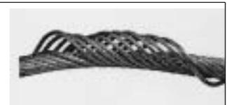
**15** Protrusion of rope centre resulting from build up of turn.
