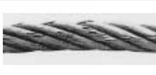
**5** Severe wear, associated with high tread pressure.
