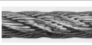
**3** Narrow path of wear resulting in fatigue fractures, caused by working in a grossly oversize groove, or over small support rollers.
