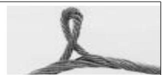
**16** Substantial wear and severe internal corrosion.
